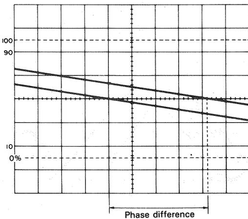
Expanded sweep waveform display.
